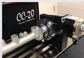
Programmable Motorized Rotary Indexer for staging shafts and cylinders.
