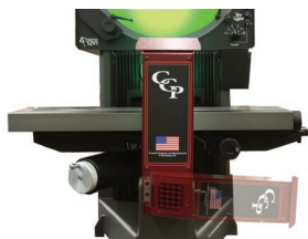
Swing Away Lamphouse allows oversized parts to be staged.
